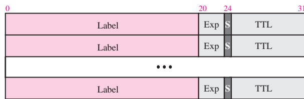
Figure 6.21 MPLS header made of stack of labels
