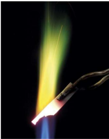
Copper being burnt in a flame from a Bunsen burner. Copper burns with a green/blue flame in the presence of oxygen to form copper (II) oxide
