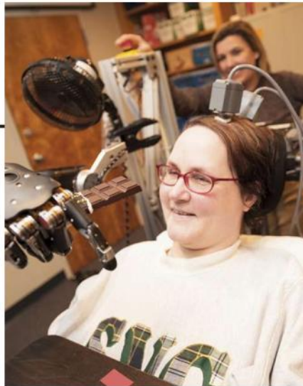
Quadruplegic Jan Scheuermann uses thought to control a robotic arm
