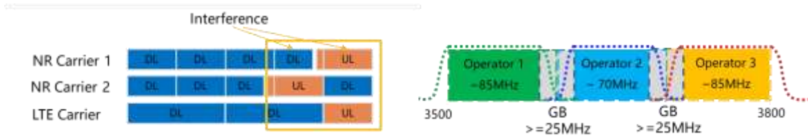
Figure 15: 4:1 and 8:2 time slot configuration
